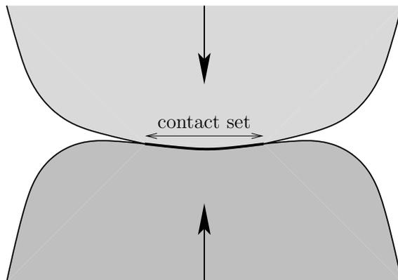
Figure 7.1: Definition sketch for contact between two solids.
