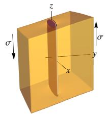
Crack along x-axis subject to shear stress σ in z-direction.
