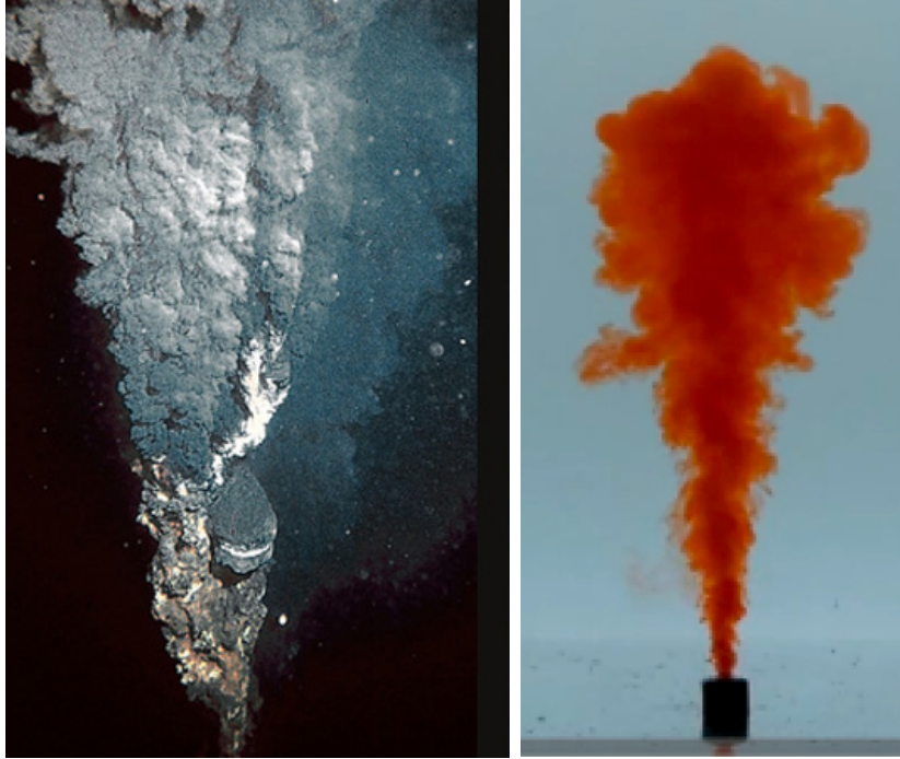
Figure 3.13: On the left, a sub-oceanic black smoker issuing from a vent at the ocean floor; image from http://oceanexplorer.noaa.gov . On the right, a laboratory plume; image courtesy of Andy Woods.
