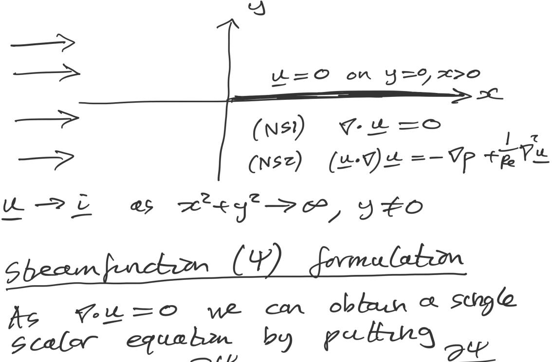
$u = \frac{\partial u}{\partial y}$  and  $v = -\frac{\partial u}{\partial x}$ . [Watch Ele sign convention.] Now ne con éliminate the pressure p by forming the vortitity equation for  $\omega = -\nabla^2 \Psi$ .  $(\underline{u}, \overline{v})(\overline{v}^{2} \Psi) = \Psi_{y} \overline{v}^{2} \Psi_{z} - \Psi_{z} \overline{v}^{2} \Psi_{y}$  $= \frac{1}{Re} \nabla^2 \left( \nabla^2 \Psi \right)$ since  $\exists_y(\exists_x) = \exists_z(\exists_y).$
