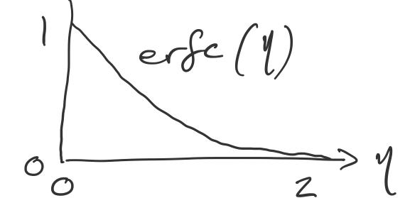
Vizcous boundary layer on a Geni-infinite plate. A noulinear problem
