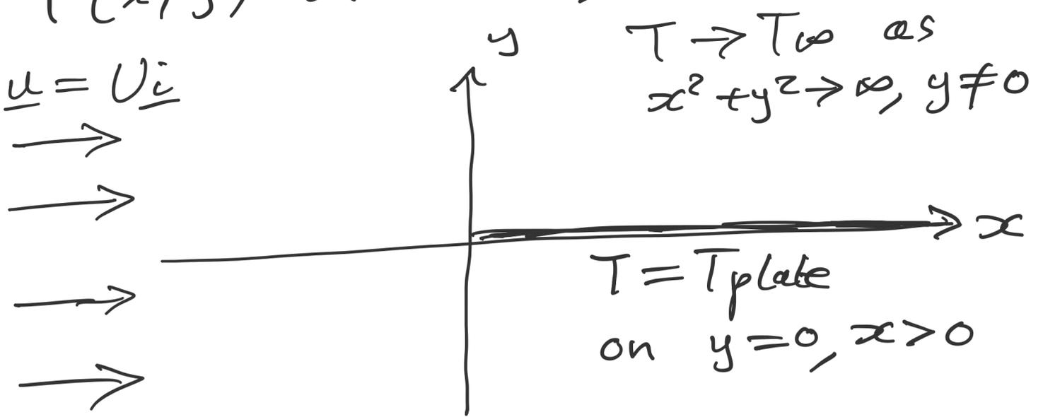
The flow, being inviscid, is undisturbed by the plate,  $\underline{u} = U \underline{i}$  everywhere.
