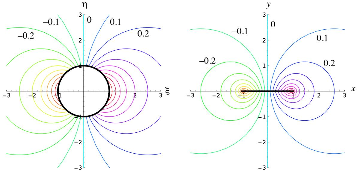
Figure 22: Contour plots of the solution  $u$  given by (318) versus  $\xi = \Re(\zeta)$  and  $\eta = \Im(\zeta)$  (left plot);  $x$  and  $y$  (right plot). The contour values are  $u = -0.9, -0.8, \dots, 0.8, 0.9$ .
