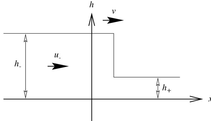
Figure 18: Schematic of a bore (with  $u_+ = 0$ ).
