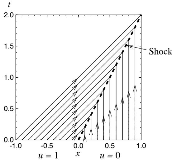
Figure 10: The characteristic projections and shock for Example 14.
