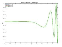
Remedy: use a large timestep when the solution does not change rapidly and a small timestep when it does.
