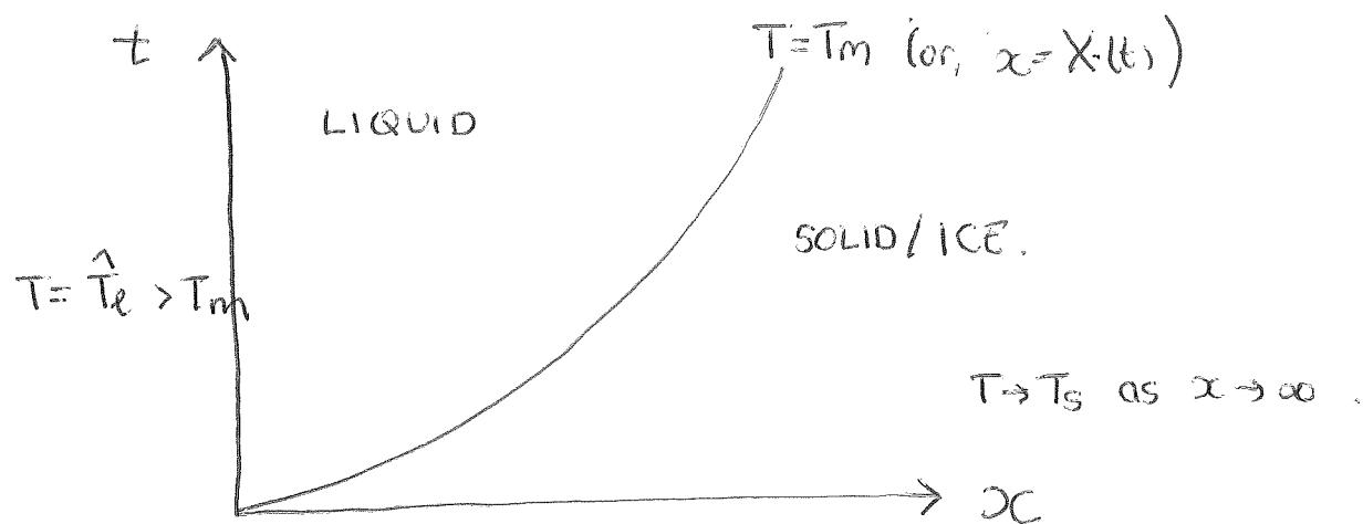
LIQUID :  $\frac{\partial T_e}{\partial t} = \alpha_e \frac{\partial^2 T_e}{\partial x^2}$        $\alpha_e = k_e / \rho c_e$ .
