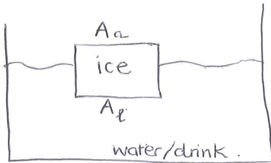
$A_a, A_e = \text{SA}$  of exchange with atmosphere & liquid.
