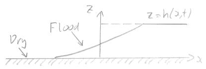
· Equivalent to piston pulling problem in gas dynamics with instantaneous piston withdrawal - hence can set 8 = 2 in solution from last Lecture!
