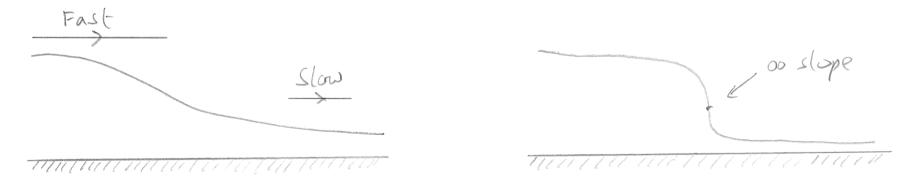
· To avoid a multi-valued solution for t> te, we must introduce a shock.
