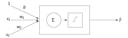
In each unit we compute a weighted sum  $z = b + w_1x_1 + w_2x_2$  and then compute a nonlinear function of z (often a sigmoid, e.g.  $a = \sigma(z)$ ).
