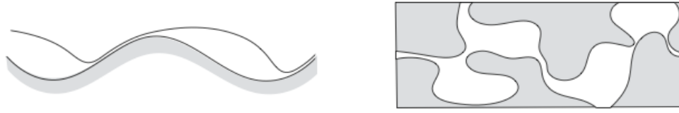
Figure 3.3: Cavitation behind bumps in bedrock viewed from the side and from above.
