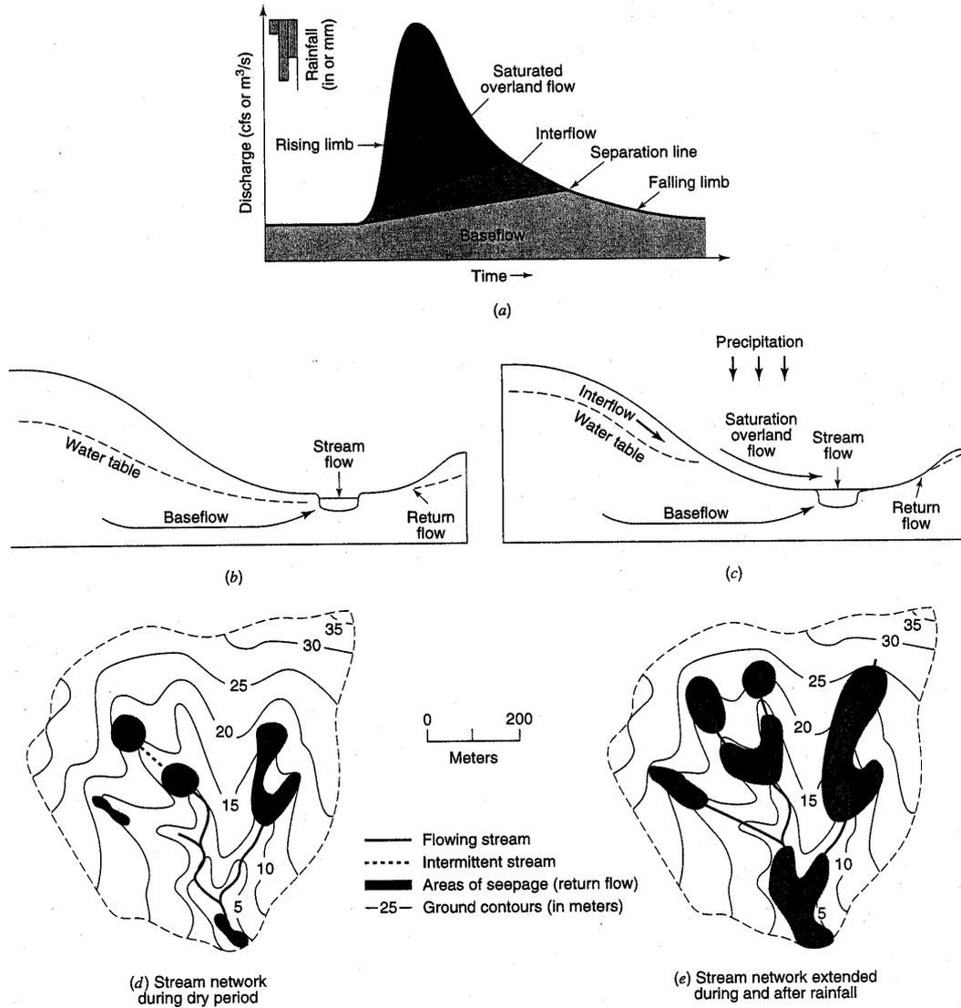
**Figure 2.1.** (a) Separation of sources of streamflow on an idealized hydrograph; (b) Sources of streamflow on a hillslope profile during a dry period; (c) During a rainfall event; (d) Stream network during a dry period; (e) Stream network extended during and after rainfall (from Mosley and McKerchen, 1993)
