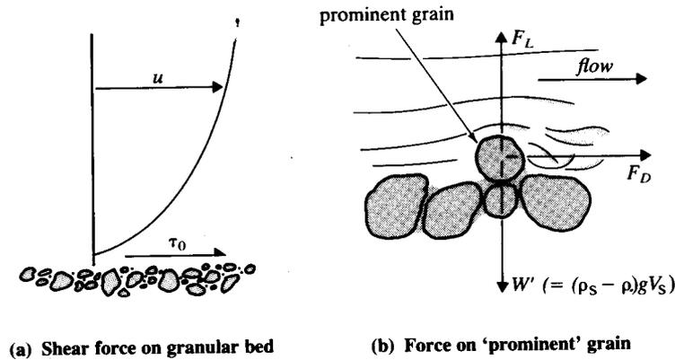
**Figure 5.** Fluid forces causing sediment movement
