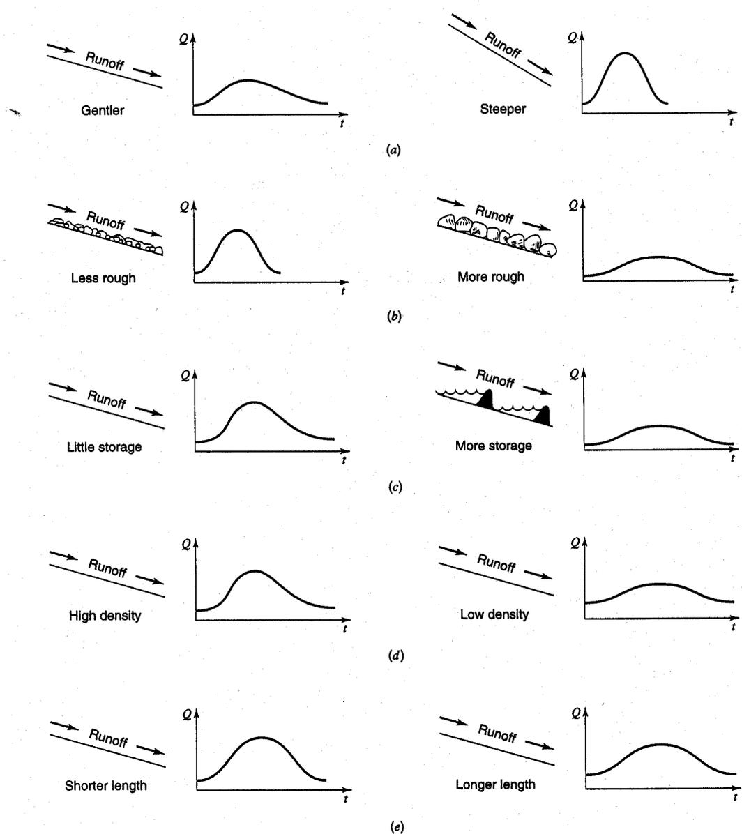
**Figure 2.2.** Effects of basin characteristics on the flood hydrograph. (a) Relationship of slope to peak discharge; (b) Relationship of hydraulic roughness to runoff; (c) Relationship of
