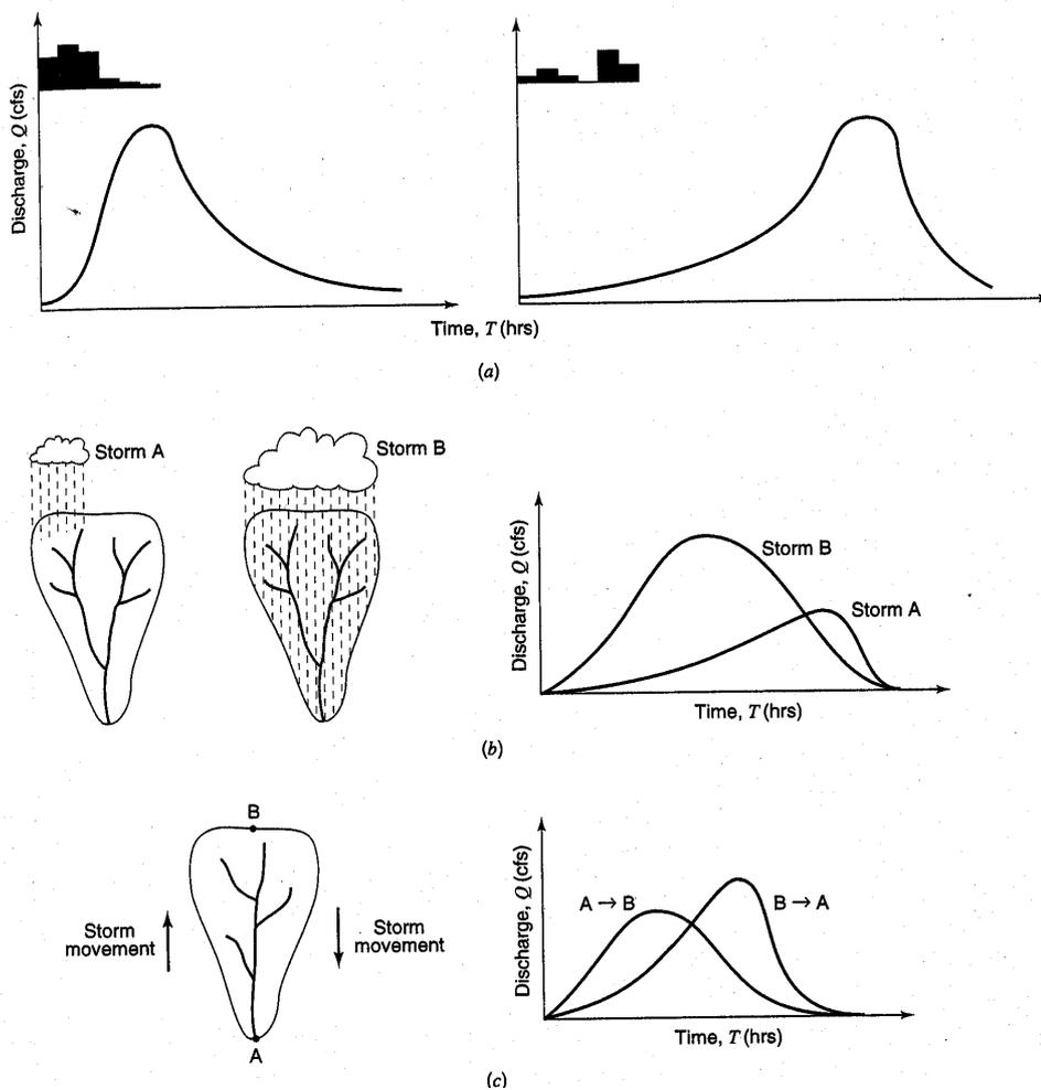
**Figure 2.3.** Effects of storm shape, size and movement on surface runoff. (a) Effect of time variation of rainfall intensity on runoff; (b) Effect of storm size on runoff; (c) Effect of storm movement on surface runoff (from Masch 1984)
