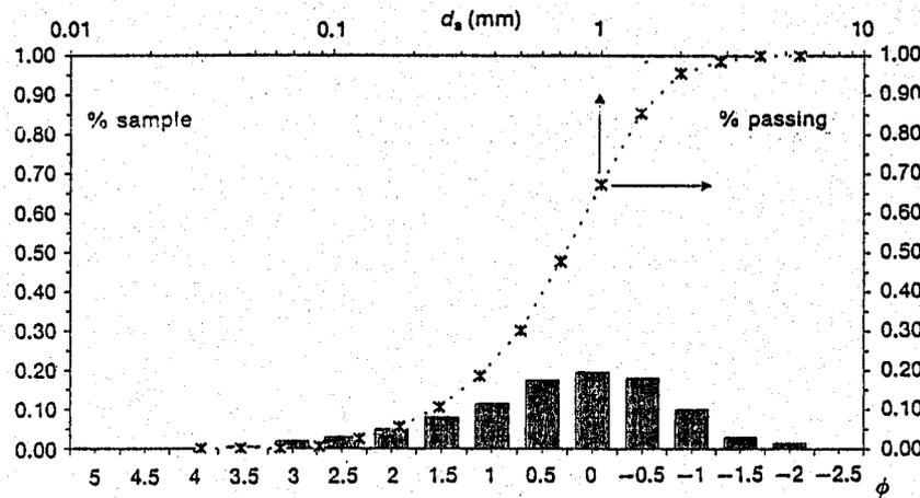
**Figure 1.** Typical particle size distribution curve. (a) Percentage sampling as a function of sedimentological size parameter  $\phi$  (linear scale). (b) Cumulative percentage passing as a function of the particle size  $d_s$  in mm (semilog scale).
