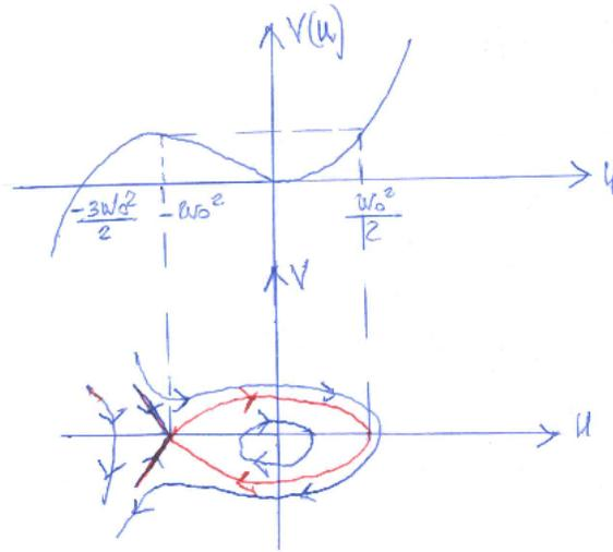
Figure 5: Sketch of the potential  $V(u)$  and the phase plane for system (29)-(30) with  $\varepsilon = 0$ .
