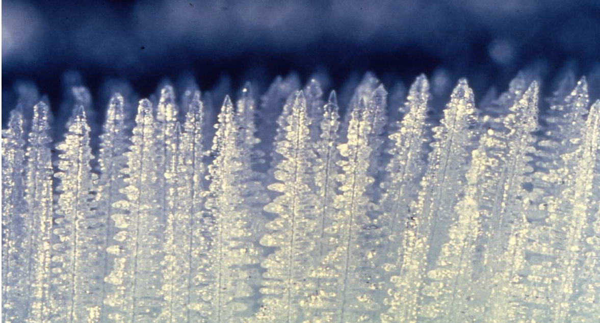
Figure 3.4: A dendritic mush in the solidification of ammonium chloride in the laboratory. Convection occurs within the mush, leading to the formation of ‘chimneys’ which act as sources of plumes in the residual melt. Photo courtesy of Grae Worster.
