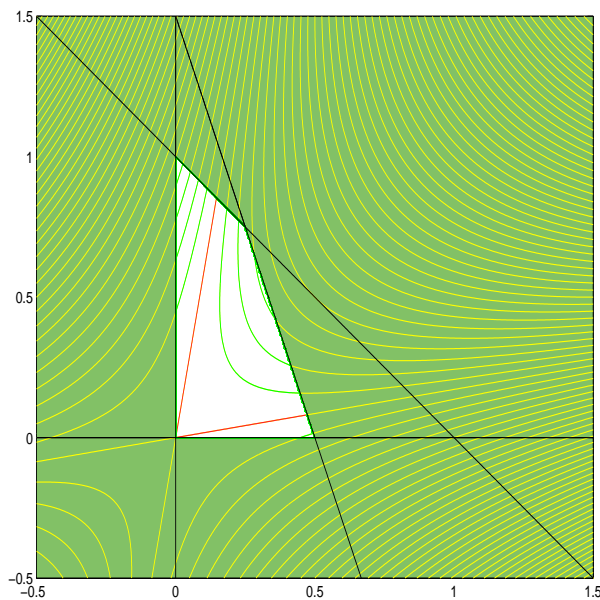
Figure 4.2: Another non-convex problem: contours of the objective function x_1^2 + x_2^2 - 6x_1x_2 and the feasible region for the constraints x_1 + x_2 \leq 1 , 3x_1 + x_2 \leq 1.5 and (x_1, x_2) \geq 0 . Note that escaping from the origin may be difficult!
