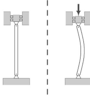
Figure 9: Buckling of a planar compressed pinned-pinned rod.
