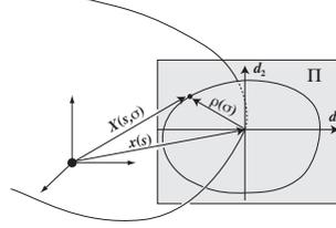
Figure 7: Cross-section of a rod and local coordinates
