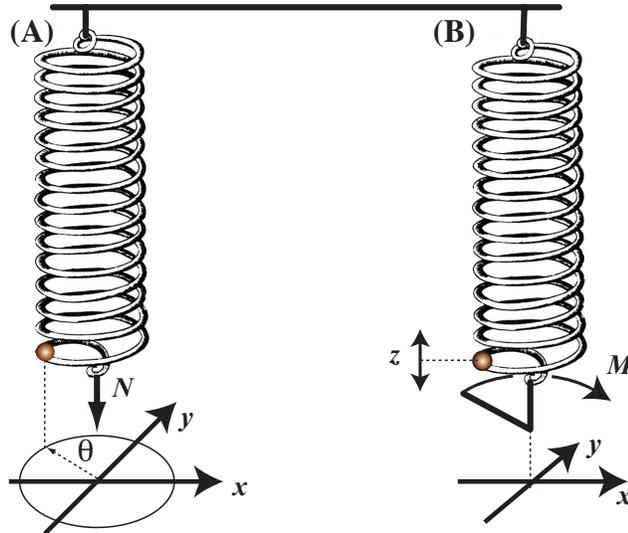
Figure 10: A wrench applied to a helical spring gives rise to another helical equilibrium. Two simple questions are to determine: (A) the sign of the increment of the rotation angle  $\theta$  when an axial tension is applied with no torque, and (B) whether a spring extends or contracts as a result of a axial torque loading with no applied force. Drawings adapted from those of Robert Hooke's 1678 Lectures De Potentia Restitutiva
