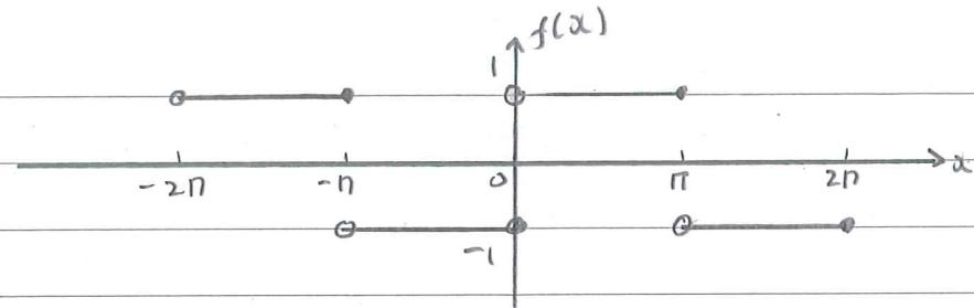
$$f \text{ odd for } x \neq kn, k \in \mathbb{Z} \Rightarrow a_n = 0, b_n = \frac{2}{\pi} \int_0^{\pi} f(x) \sin(nx) dx$$
