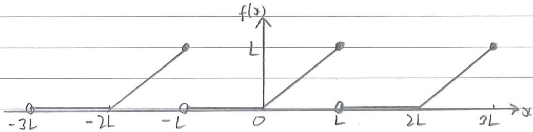
$$a_n = \frac{1}{L} \int_0^L x \cos\left(\frac{n\pi x}{L}\right) dx, \quad b_n = \frac{1}{L} \int_0^L x \sin\left(\frac{n\pi x}{L}\right) dx$$
