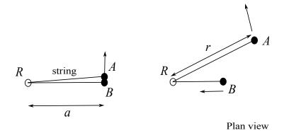
They are connected by a light inextensible string of length 2a which passes through a light ring R fixed in the table at a distance a from the particles. The ring is smooth and can rotate freely. The particle A is given an initial velocity perpendicular to the string in the plane of the table.
