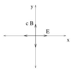
a wave like this is said to be lineary polarised;  $\vec{E}$  and  $\vec{B}$  oscillate parallel to two fixed orthogonal directions.
