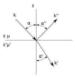
For z > 0 the solution corresponds to the incident plus the reflected waves
