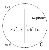
Now, lets turn out to the more interesting situation t > t'. In this case we can compute the integral over  $\omega$  by closing the contour from below. By residue theorem we obtain
