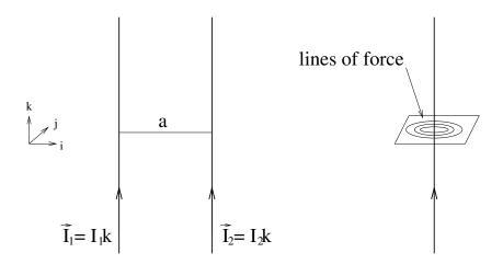
To see (127) in action, let us consider the force between two parallel current-carrying wires.
