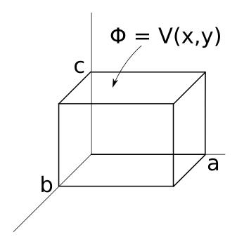
Requiring the potential to vanish at x = 0, y = 0 and z = 0 we see the potential should be the sum of terms of the form
