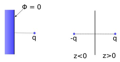
Let us locate the charge at (0,0,d) for simplicity. The method of images consist on adding *image* charges *outside* the region of interest in such a way that the boundary conditions are satisfied. The potential is then the sum of the potentials for the point charge (or charges) and their images. In the present case, it is enough to add a single image charge located at (0,0,-d) and of magnitude -q. The total potential is
