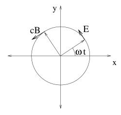
The direction is anti-clockwise and the wave is *left circularly polarized* if  $\vec{e}_1 \wedge \vec{e}_2 \cdot \vec{k} > 0$ , and the rotation is clockwise and the wave is *right circularly polarized* if  $\vec{e}_1 \wedge \vec{e}_2 \cdot \vec{k} < 0$ .
