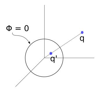
Let us denote the vector position of the point charge as  $\vec{r}_q = \mathbf{n}_q b$  and let us assume that only one image charge of magnitude q' is enough. By symmetry, the image charge should lie on the ray from the origin to the original point charge. The scalar potential would then be
