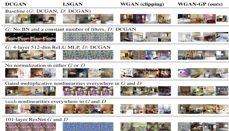
Figure 2: Different GAN architectures trained with different methods. We only succeeded in training every architecture with a shared set of hyperparameters using WGAN-GP.
