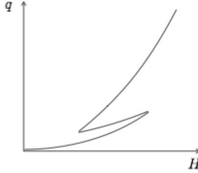
Figure 3.5: Multivalued relationship between ice thickness and flux.
