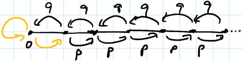
$$\begin{aligned} p_{i,i+1} &= p \\ p_{i,i-1} &= q = 1-p \end{aligned} \quad \left\{ \begin{array}{l} i \geq 1, \text{ for } p \in (0,1) \end{array} \right.$$
