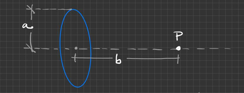
Find E at a point P on the axis of the circle at a distance 6 from the antiWe will do this directly from conlomb's law by arting the wire into small elements and then us the superposition principle to add up all the comprised butions.
