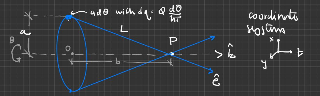
constribution to  $\vec{E}$  at  $\vec{P}$  of dq  $= \frac{1}{4\pi 60}$   $\vec{Q} d\theta (18)$ ,  $L^2 = a^2 + b^2$ Note that the components property color to the tractis of diametrically opposite wire segments cancel each other ! Thus, a dding all contributions around the circle  $\vec{E} = \vec{E} \cdot \vec{b} \cdot \vec{s} \cdot \vec{s}$  $\vec{b} \cdot \vec{E} \cdot \vec{s} \cdot \vec{s}$
