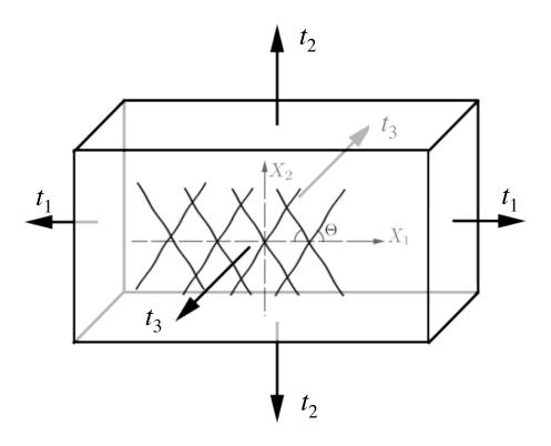
Figure 25: A cuboid is subjected to external hydrostatic loading, maintaining constant normal stress on each face of the cuboid. The material is reinforced by two families of fibers, which are in-plane, aligned symmetrically, and make an angle  $\Theta$  with the  $\mathbf{E}_1$  direction.
