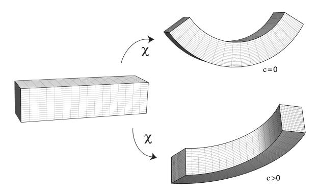
Figure 17: Family 1. Bending, stretching, and shearing of a rectangular block. When the parameter c vanishes, the deformation corresponds to the bending/stretching of a block. The parameter c is associated to shearing out of the bending plane.
