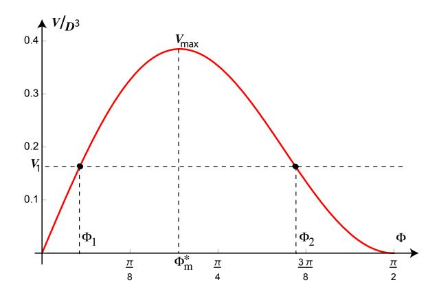
Figure 34: The magic angle gives the maximal enclosed volume of a cylinder reinforced by inextensible fibers of fixed length D. For  $V < V_{\text{max}}$  there exist two angles at fixed volume.
