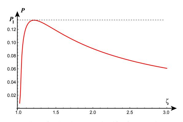
Figure 14: Behavior of a tube under pressure and axial force for a Neo-Hookean material  $(A = 1, B = 1.2, \mu = 1, F = 0.1, \chi = 1)$ . The neo-Hookean model is ill defined past a critical pressure  $P_1$ .
