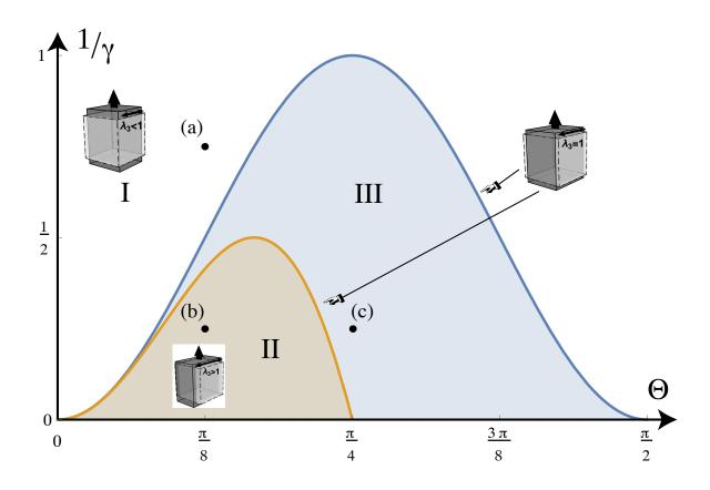
Figure 29: Parameter space for inversion: depending on the relative fiber stiffness  $\gamma$  and the fiber direction  $\Theta$ , in tension, the thickness of a either decreases (Zone I), increases (Zone II), or first decreases, then increases (Zone III). Insert shown for different values of the tension. The stretch profiles as a function of the tension for specific points (a,b,c) are given in Figure 28.
