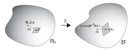
Figure 7: Transformation of area: In a deformation, an infinitesimal area is transformed according to Nanson's rule.
