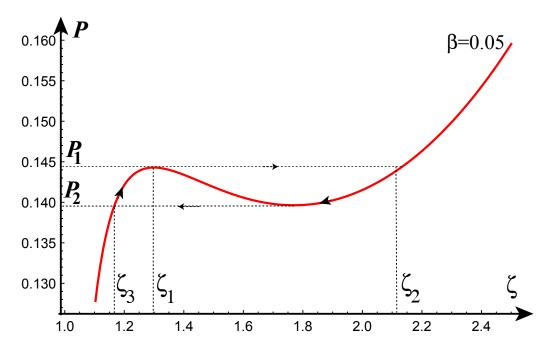
Figure 16: Limit-point instability in of a tube under pressure and axial force for a Fung material ( $\beta = 0.05$ ). The curve  $P(\zeta)$  has a minimum and a maximum. If the internal pressure of the tube is raised to  $P_1$ , a sudden extension occurs through a jump from  $\zeta_1$  to  $\zeta_2$ . When the pressure is then decreased to  $P_2$ , a second jump occurs to  $\zeta_3$  (lower arrow).
