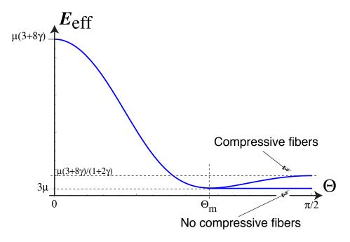
Figure 27: Effective Young's modulus for a fiber-reinforced sheet as a function of the fiber angle.
