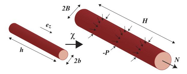
Figure 13: Inflation-extension of a tube. The tube is inflated with an internal pressure P (which is equivalent to an external pressure -P as shown) and an axial load N resulting from an applied load and the pressure acting on the end caps.
