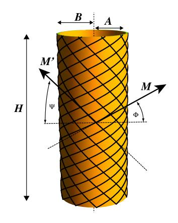
Figure 30: Geometry of the fibers. The angle  $\Phi$  denote the direction of the first fiber with respect to the cross section (counted counter-clockwise) and the angle  $\Psi$  is the angle of the second fiber (counted clockwise).
