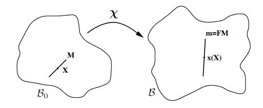
Figure 24: A one-fiber material. In an anisotropic one-fiber material, the response of the material depends on the deformation gradient  $\mathbf{F}$  and the direction of a distinguished material line represented by a unit vector  $\mathbf{M}$ . In a deformation, this direction is mapped to a vector  $\mathbf{m} = \mathbf{F}\mathbf{M}$ .
