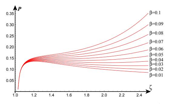
Figure 15: Behavior of a tube under pressure and axial force for a Fung material ( $\beta > 0$ ). Parameters for all figures:  $A = 1, B = 1.2, \mu = 1, F = 0.1, \chi = 1$ .
