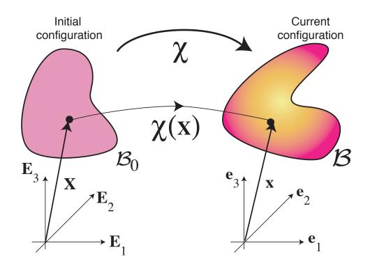
Figure 3: Basic kinematic of nonlinear elasticity. Two configurations are defined. The deformation is a 1-1 map between points of the reference configuration  $\mathcal{B}_0$  and points of the current configuration  $\mathcal{B}$ .
