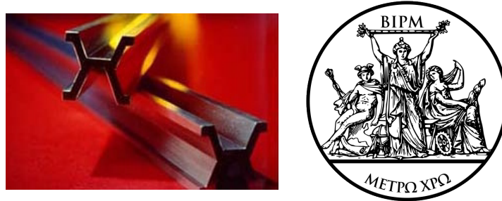
Figure 1: The cross-section shape of the metre bar is an X-shape. Why? What is BIPM?
