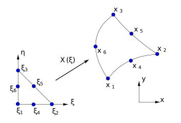
Figure 9.3: It is possible to represent the coordinate field with Lagrange elements of higher order, allowing us to bend the mesh. This is useful if  $\Omega$  is not a polygon or polyhedron.
