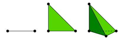
Figure 1.4: The linear Lagrange element in one, two and three dimensions. The black circles denote pointwise evaluation. These pictures describe what values need to be stored to define a function on the cell.
