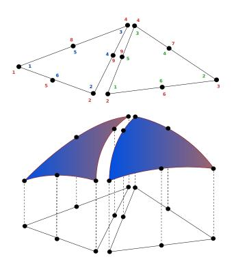
Figure 8.3: The local-to-global mapping for a simple mesh consisting of two triangles, both equipped with secord order Lagrange elements. By mapping matching local degrees of freedom at the common edge to the same global degree of freedom, the local-to-global map ensures the  $C^0$  continuity of the approximation.
