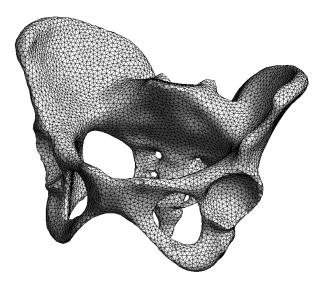
Figure 1.2: A mesh of a human pelvis, produced using the gmsh software.
