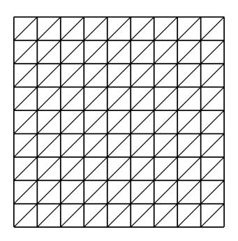
Figure 14.1: The mesh on which we will construct a spurious pressure mode.
