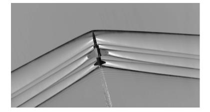
Figure 1.1: A supersonic aircraft induces a shock wave; physical reality is best described by a discontinuous function. The blurring of the interface is an artefact of an averaging process in the photography; the true interface is sharper. Credit: https: //www.nasa.gov/centers/armstrong/ features/shock\_and\_awesome.html
