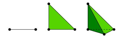
**Example 8.1.2.** Consider the standard linear Lagrange finite element on the triangle, figure 8.1. The cell K is given by the triangle and  $\mathcal{V}$  is the space of first degree polynomials on K (a space of dimension d = 3). As a basis for
