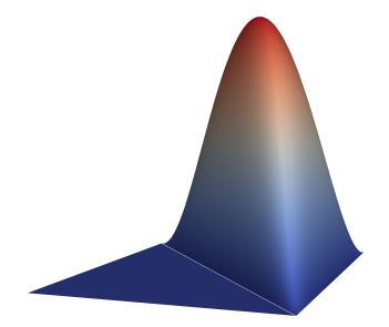
Figure 10.4: The Hermite element does not guarantee a  $C^1(\Omega)$  discretisation in two dimensions. The function (10.2.12) is in the Hermite space but its normal derivative is not continuous at the shared edge.
