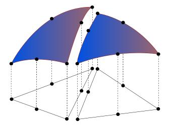
Figure 8.4: By *not* mapping matching local degrees of freedom at the common edge to the same global degree of freedom, a discontinuous approximation results.
