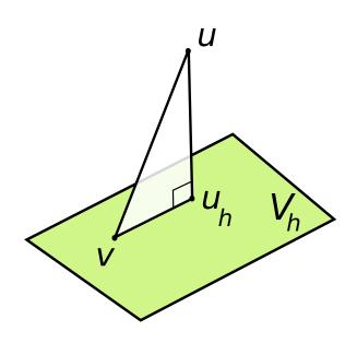
Figure 7.1: For symmetric problems, the Galerkin approximation is the orthogonal projection of the solution onto the trial space when measured in the energy norm. Credit: Oleg Alexandrov, Wikipedia.
