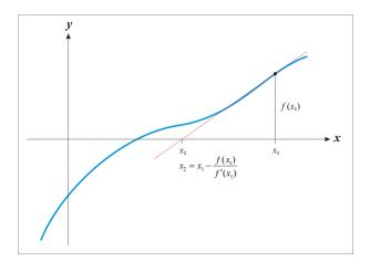
Figure 12.1: Each iteration of Newton's method consists of linearising the nonlinear problem and solving for the root of the linearised problem. Credit: Ralf Pfeifer, Wikipedia.
