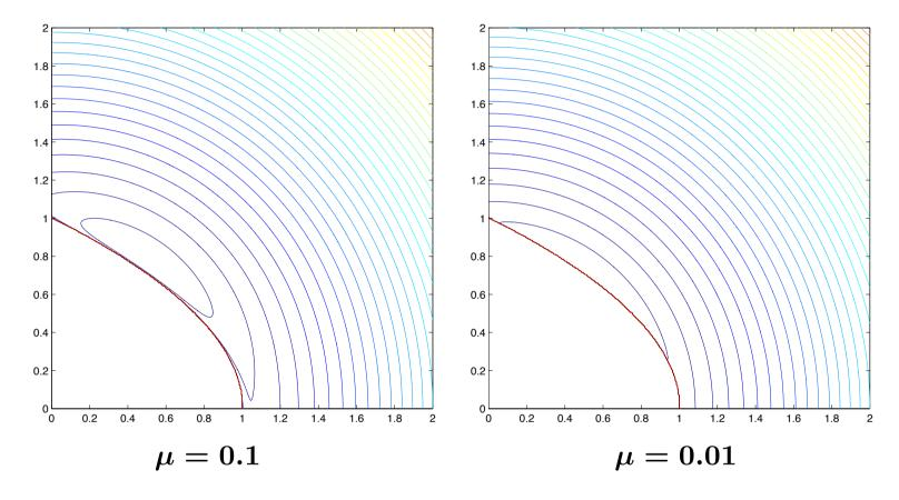
The barrier function for  $\min x_1^2 + x_2^2$  subject to  $x_1 + x_2^2 \ge 1$ ,  $f_\mu(x) := x_1^2 + x_2^2 - \mu \log(x_1 - x_2^2 - 1).$
