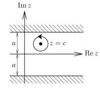
Figure 4.3: Schematic of a vortex in the channel -a < Im z < a.
