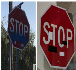
Figure 1: The left image shows real graffiti on a Stop sign, something that most humans would not think is suspicious. The right image shows our a physical perturbation applied to a Stop sign. We design our perturbations to mimic graffiti, and thus “hide in the human psyche.”
