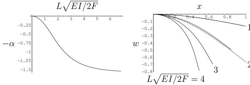
Figure 6.7: (a) Final angle  $-\alpha$  of a diving board versus applied force parameter  $L\sqrt{2F/EI}$ . (b) Deflection of a diving board for various values of the force parameter; the dashed lines show the linearised solution.
