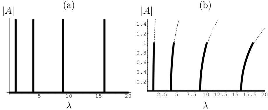
Figure 6.8: (a) Response diagram of the amplitude  $\|\theta\|$  of the linearised solution (6.39) for a buckling beam versus the force parameter  $\lambda$ . (b) Corresponding response of the weakly nonlinear solution; the exact nonlinear solution is shown using dashed lines.
