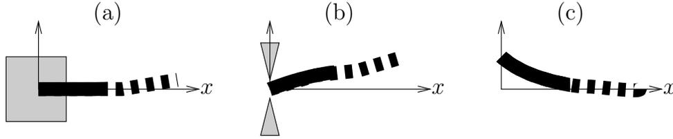
Figure 6.4: Schematic of the end of a beam under (a) clamped, (b) simply supported and (c) free conditions.
