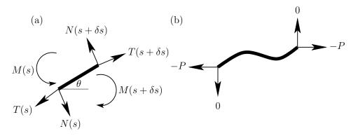
(a) Balance forces and moments on a small segment of the beam as shown in (a) above, neglecting inertia and body forces to get
