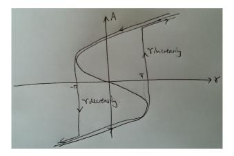
When  $\gamma$  starts at  $-2\pi$ , the solution starts on the lower branch with  $A_1$  negative and the beam bending downwards. As  $\gamma$  increases through the critical value  $\pi$ , the beam "snaps through" to the other branch where  $A_1 > 0$  and the beam bends upwards. As  $\gamma$  then decreases it stays on the upper branch until  $\gamma = -\pi$  when it then snaps back onto the lower branch again.
