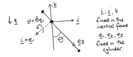
(c) The above cylinder swings in a vertical plane, hinged at a point half way between an end of the cylinder and its centre of mass. Let  $\theta(t)$  denote the angle from the downward vertical to the longer segment of the cylinder, of length 3l/4. Show that the equation of motion for the cylinder is given by
