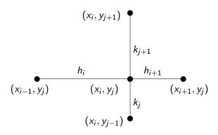
Figure: Five-point stencil on a non-uniform mesh.
