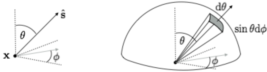
Figure 1.2: Radiative intensity is a function of position \mathbf{x} and direction \hat{\mathbf{s}} = (\sin \theta \cos \phi, \sin \theta \sin \phi, \cos \theta) . An element of solid angle has projected area on the unit sphere d\omega = \sin \theta d\theta d\phi .
