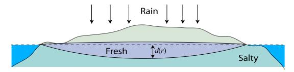
Consider a permeable island situated within a salty body of water (as illustrated in the figure above). Because of the infiltration of fresh (rain) water of density  $\rho_0$  at a constant flux  $w_r$  per unit area a lens of fresh water forms 'floating' above and displacing the more dense salt water (density  $\rho_s$ ) that permeates the porous medium beneath sea level.
