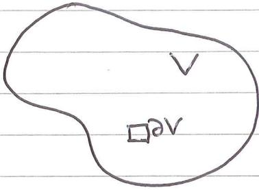
Let  $c(\underline{x}, t)$  be the amount of heat (or chemical) per unit vol. at position  $\underline{x}$  & time  $t$ .
