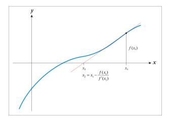
Figure 12.1: Each iteration of Newton's method consists of linearising the nonlinear problem and solving for the root of the linearised problem. Credit: Ralf Pfeifer, Wikipedia.
