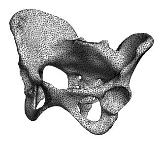
Figure 1.2: A mesh of a human pelvis, produced using the gmsh software.
