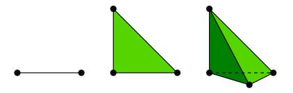
**Example 8.1.2.** Consider the standard linear Lagrange finite element on the triangle, figure 8.1. The cell K is given by the triangle and V is the space of first degree polynomials on K (a space of dimension d = 3). As a basis for
