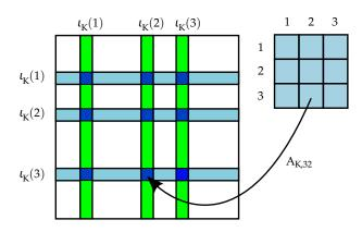
Algorithm 9.1.2: The efficient algorithm for assembly.
