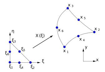
Figure 9.3: It is possible to represent the coordinate field with Lagrange elements of higher order, allowing us to bend the mesh. This is useful if  $\Omega$  is not a polygon or polyhedron.
