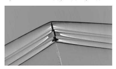
Figure 1.1: A supersonic aircraft induces a shock wave; physical reality is best described by a discontinuous function. The blurring of the interface is an artefact of an averaging process in the photography; the true interface is sharper. Credit: https://www.nasa.gov/centers/armstrong/
