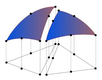
Figure 8.4: By *not* mapping matching local degrees of freedom at the common edge to the same global degree of freedom, a discontinuous approximation results.
