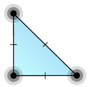
Figure 10.5: The Argyris element in two dimensions is  $C^1(\Omega)$ -conforming, and thus is  $H^2(\Omega)$ -conforming. The degrees of freedom are evaluation of the zeroth, first and second derivatives at the vertices, plus evaluation of the normal derivative at the midpoint of the edges.
