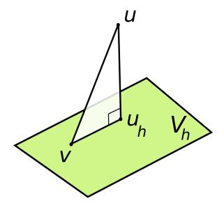
Figure 7.1: For symmetric problems, the Galerkin approximation is the orthogonal projection of the solution onto the trial space when measured in the energy norm. Credit: Oleg Alexandrov, Wikipedia.
