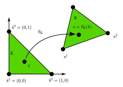
Figure 9.2: The finite element for a specific cell of the mesh *K* can be constructed via a map  $F_K$  applied to an abstract reference element  $\hat{K}$ .
