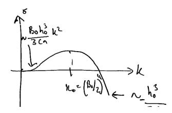
We see that the surface tension term  $(-k^4)$  is stabilising since it makes  $\sigma$  more negative, while gravity  $(+\text{Bo }k^2)$  is destabilising since it acts to increase  $\sigma$ .
