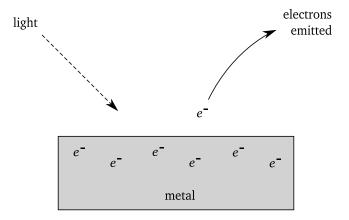
Figure 1: To observe the photoelectric effect, light is shone on a metal plate in vacuum. Electrons  $e^-$  are emitted from the surface of the metal, and their kinetic energy  $E_{\rm kinetic}$  is measured.
